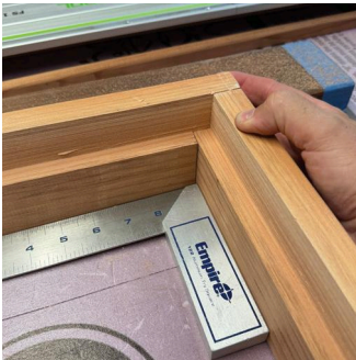
Joining jamb pieces.
